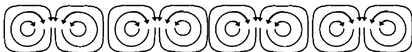
FIG. 1. Schematic of a chain of alternating vortices. The arrows show the direction of the flow within each vortex.
